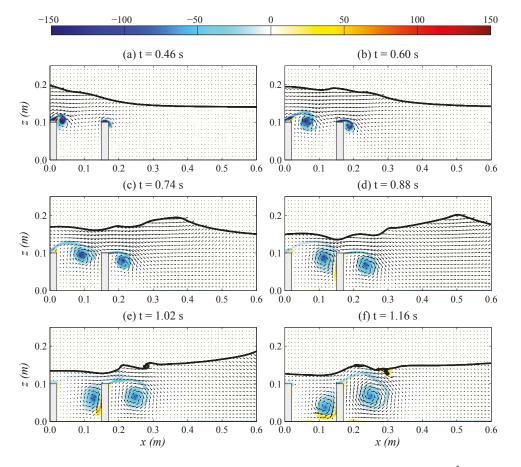
the weather side of the second barrier, which may lead to the instability issue on the foundation of the second barrier.
