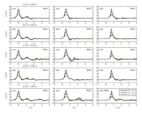
**Figure 3.** Model–data comparison in terms of free surface time series recorded by WG1, WG2 and WG3, for the cases of: (**a**) D = 0.00 m; (**b**) D = 0.05 m; (**c**) D = 0.15 m; (**d**) D = 0.35 m; and (**e**) D = 1.00 m. The solid lines and dashed lines correspond to the numerical and measured results, respectively.
