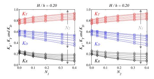
**Figure 11.** Effects of  $N_1$  with respect to  $N_2$  (left column) and  $N_2$  with respect to  $N_1$  (right column) on the hydraulic performance, for the case of H/h = 0.20. Black, red and blue colors represent  $K_R$ ,  $K_T$  and  $K_D$ , respectively.
