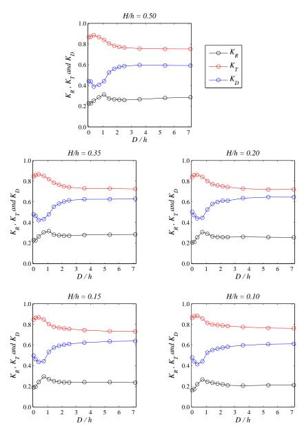
**Figure 8.** Effects of the horizontal distance (*D*) between two barriers on the energy reflection ( $K_R$ ), transmission ( $K_T$ ) and dissipation ( $K_D$ ) coefficients, for the cases of H/h = 0.50, 0.35, 0.20, 0.15 and 0.10.
