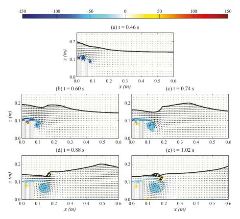
**Figure 5.** Simulated evolutions of the free surface elevation, velocity and vorticity (unit:  $s^{-1}$ ) (color map) fields for the case of D = 0.05 m at five time instants: (a) t = 0.46 s; (b) t = 0.60 s; (c) t = 0.74 s; (d) t = 0.88 s; (e) t = 1.02 s.
