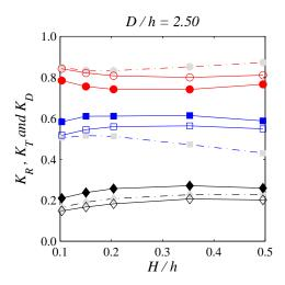
**Figure 10.** Effects of H/h on the hydraulic performance for fixed D/h = 2.50. The hollow and solid symbols respectively depict the results of  $N_1 = N_2 = 0.10$  and 0.00 scenarios. The dashed lines with gray signs show the results of single solid barrier case. Black, red and blue colors represent  $K_R$ ,  $K_T$  and  $K_D$ , respectively.
