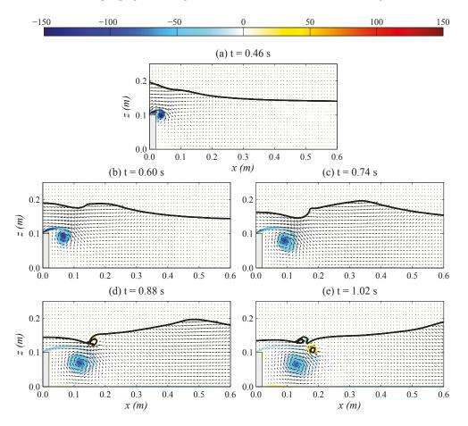
**Figure 4.** Simulated evolutions of the free surface elevation, velocity and vorticity (unit:  $s^{-1}$ ) (color map) fields for the case of D = 0.00 m at five time instants: (**a**) t = 0.46 s; (**b**) t = 0.60 s; (**c**) t = 0.74 s; (**d**) t = 0.88 s; (**e**) t = 1.02 s.
