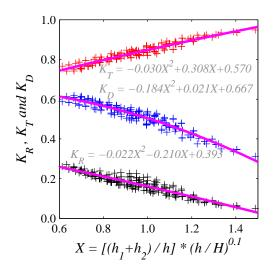
**Figure 12.** Regression analyses based on all simulations in terms of the hydraulic performance  $(h_1 = h - a \times N_1, h_2 = h - a \times N_2)$ . Symbols in black, red and blue colors represent  $K_R$ ,  $K_T$  and  $K_D$ , respectively, where the purple lines indicate the associated fitting curves for each energy coefficient.
