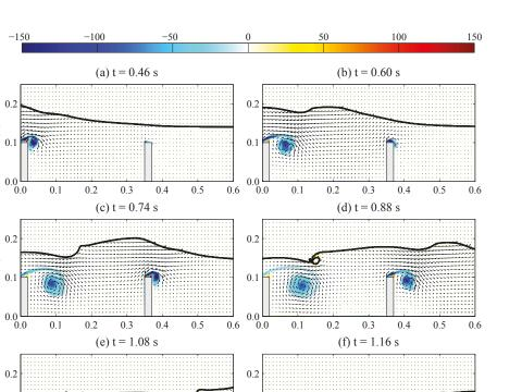
0.0 L 0.0 0.0 0.5 0.0 0.1 0.2 0.3 0.4 0.6 0.1 0.2 0.3 0.4 0.5 0.6 x(m)x(m)**Figure 7.** Simulated evolutions of the free surface elevation, velocity and vorticity (unit:  $s^{-1}$ ) (color map) fields for the case of D = 0.35 m at six time instants: (a) t = 0.46 s; (b) t = 0.60 s; (c) t = 0.74 s; (d) t = 0.88 s;
