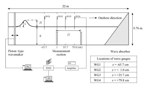
**Figure 1.** Overview of experimental set-up, facilities (not to scale) and definitions of variable assigned for a dual-solid-barrier configuration.
