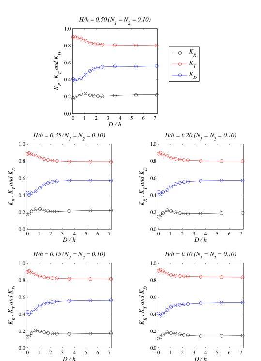
**Figure 9.** Effects of the horizontal distance (*D*) between two slotted barriers on the energy reflection ( $K_R$ ), transmission ( $K_T$ ) and dissipation ( $K_D$ ) coefficients, for the cases of H/h = 0.50, 0.35, 0.20, 0.15 and 0.10.
